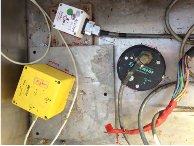
Fig. 2. 6DOF observation instruments deployed in GVDA site. The yellow box is the Eentec model R-1 rotational sensor (location code 21), the black cylinder is the Kinemetrics ES-T translational accelerometer (location code 00). (For interpretation of the references to color in this figure legend, the reader is referred to the web version of this article.)
