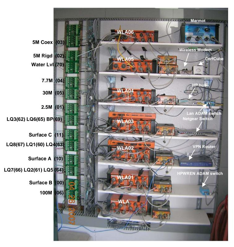
The power-supply for the sensors is routed through the +12V channels of the LP boards. IT has been found that noise from the solar charge controllers contaminates the sensor signals when used to power the sensors directly. For this reason, Acopian dc/dc bricks are being used to isolate and filter the power-supply to the sensors.
