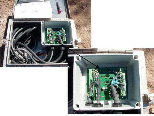
A Surface Accelerometer housed in a stainless-steel Hoffman box.
