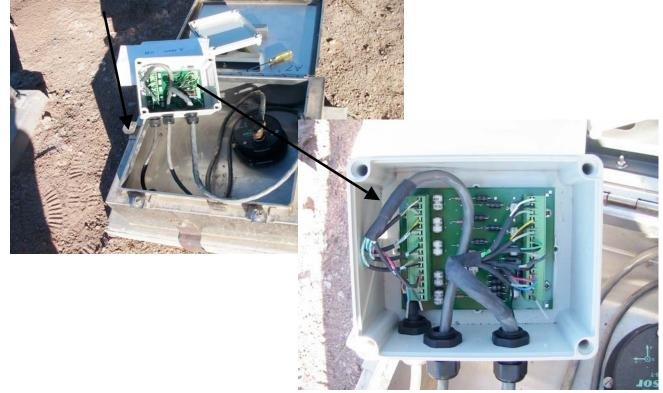
A Surface Accelerometer housed in a stainless-steel Hoffman box.
