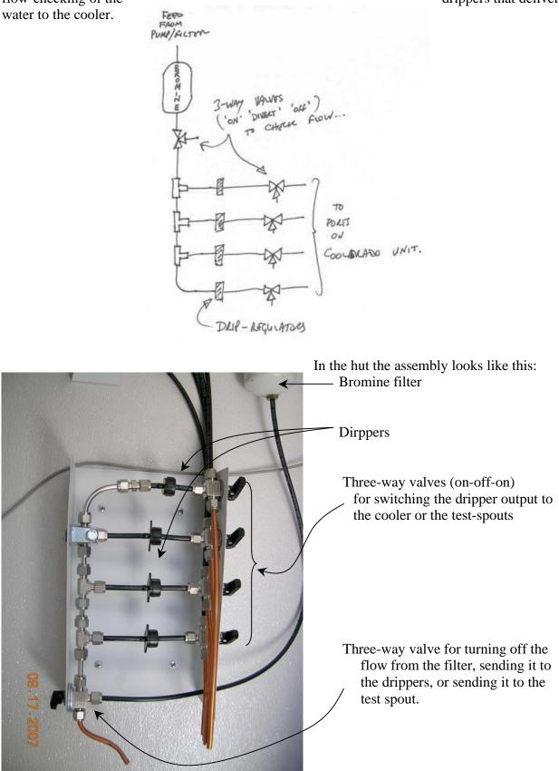
With this arrangement the water flow from the bromine filter can be checked, the flow to the dirppers can be turned off and they can be removed and replaced by way of the Swagelok compression fittings, and the flow for each of the individual dripper output can be checked inplace.
