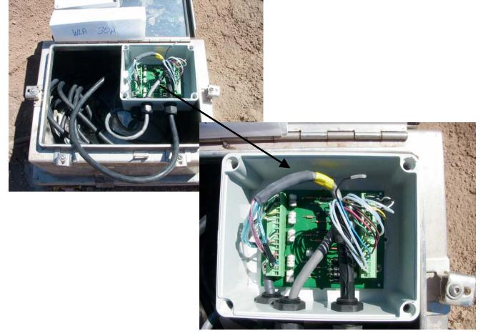
A Surface Accelerometer housed in a stainless-steel Hoffman box.
