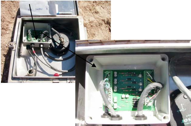
A Surface Accelerometer housed in a stainless-steel Hoffman box.
