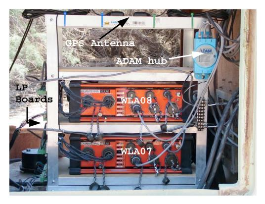
The hut is cabled to the main building with two power circuits (12 Awg pairs) and a single waterproof cat-5 network connection.
