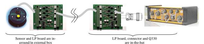
In the case above, an EpiSensor surface accelerometer with three channels is connected to a local Lightning Protection board in the wellhead box before the signals are passed through an underground cable into the hut.
