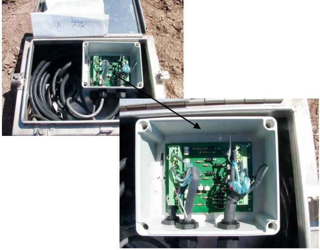
A Surface Accelerometer housed in a stainless-steel Hoffman box.
