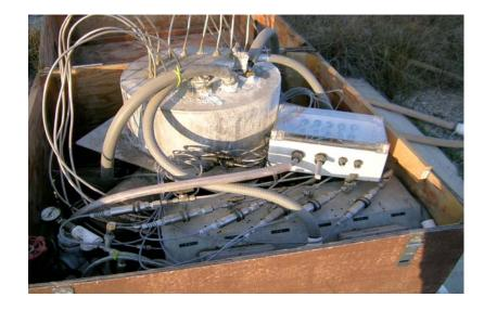
A collection of pore-pressure transducers in the 500M borehole at various depths.
