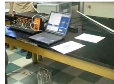
The equipment setup with laptop computer, laser printer, Q330 datalogger and accelerometer.
