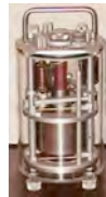
The working Geotech Instruments Model S-13 is housed in a plexiglass case.
