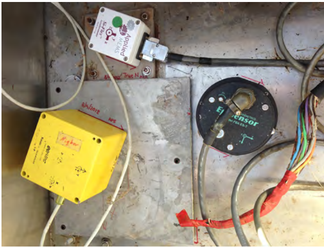
Fig. 2. 6DOF observation instruments deployed in GVDA site. The yellow box is the Eentec model R-1 rotational sensor (location code 21), the black cylinder is the Kinemetrics ES-T translational accelerometer (location code 00). (For interpretation of the references to color in this figure legend, the reader is referred to the web version of this article.)
