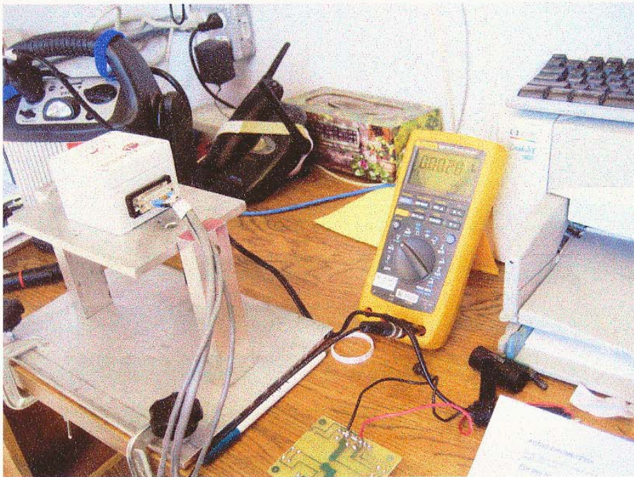
Setup for Accelerometer Tilt Calibration
