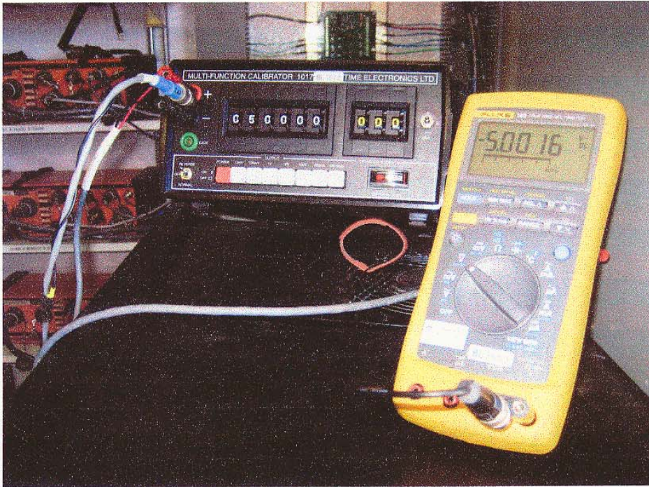
Measuring step for A/D channel check/calibration
