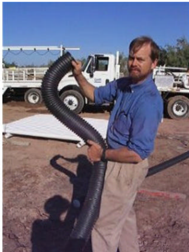
Figure 13 Rob Steller demonstrating the flexibility of flexible drain pipe installed at WLA for measurement of earthquake-induced permanent lateral ground deformations
