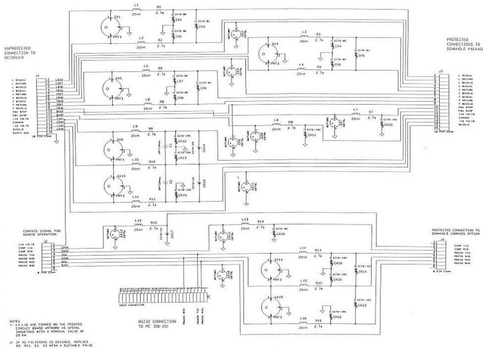
The board layout pretty much flows as drawn in the schematic, from left to right there is the three-terminal gas-discharge tube, into a series impedance (R+L) followed by the transorbs, with the last gas-discharge tube on the right protecting the 'shield' to ground.
