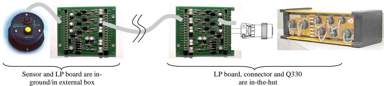
In the case above, an EpiSensor surface accelerometer with three channels is connected to a local Lightning Protection board in the wellhead box before the signals are passed through an underground cable into the hut.
