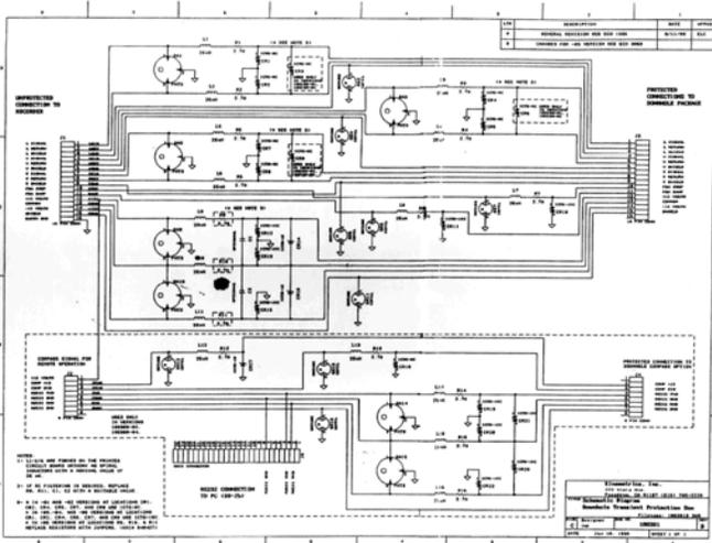
The board layout pretty much flows as drawn in the schematic, from left to right there is the three-terminal gas-discharge tube, into a series impedance (R+L) followed by the transorbs, with the last gas-discharge tube on the right protecting the 'shield' to ground.
