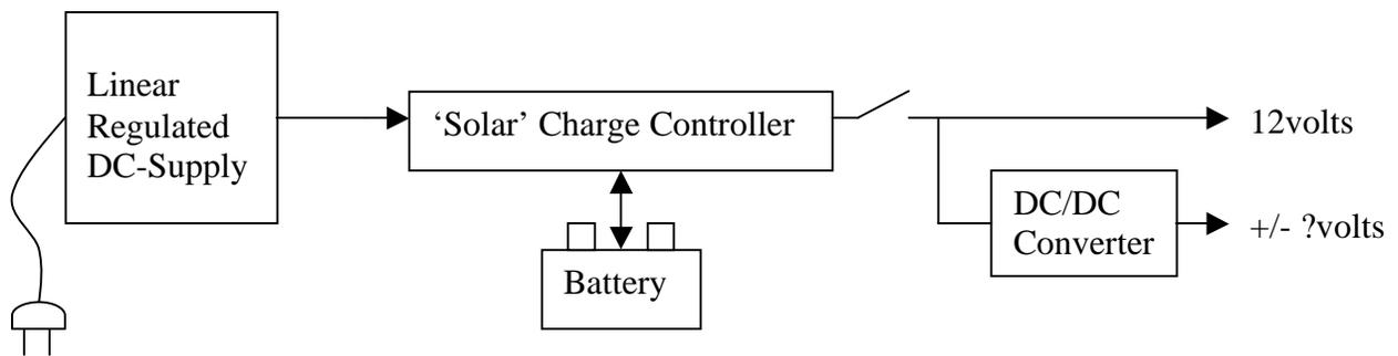
When voltages other than standard +12V are required, individual dc/dc converters are used.
