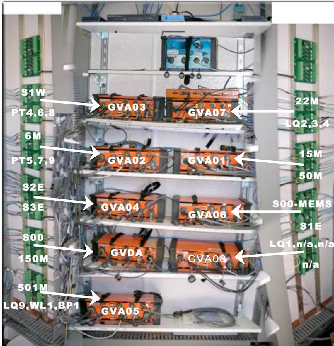
The power-supply for the sensors is routed through the +/-12V channels of the LP boards.
