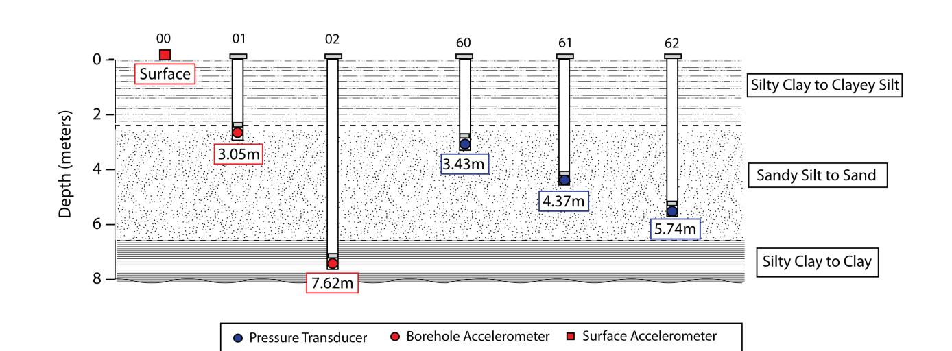
Figure 2: A cross section showing instrumentation at the NEES@UCSB Wildlife Station (Holzer and Youd, 2007, Youd et al., 2007).
