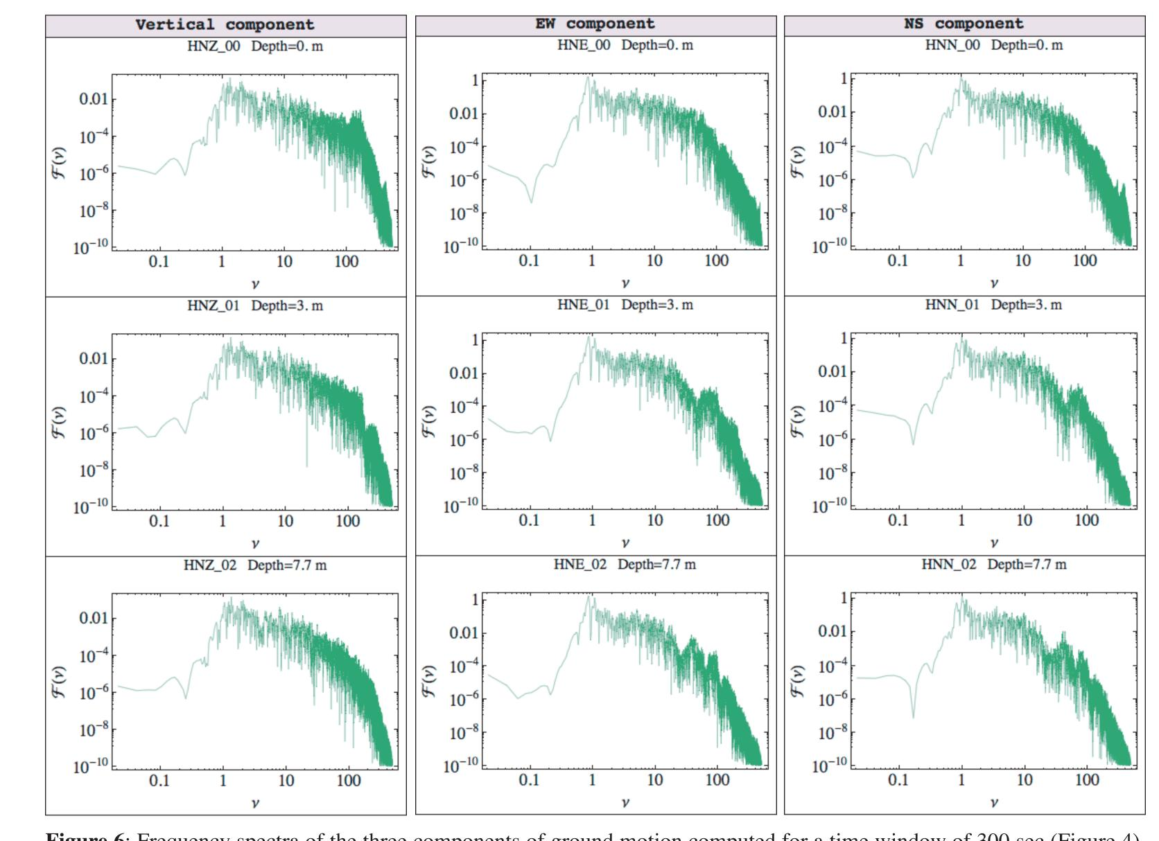
Figure 6: Frequency spectra of the three components of ground motion computed for a time window of 300 sec (Figure 4). The shapes of the curves are complicated, especially for the EW and NS components, and there is no simple functional representation. Note that for the EW and NS components at 3 m and 7.7 m depths, there are depletions of the spectral curves at several frequencies in the range 10 to 100 Hz.
