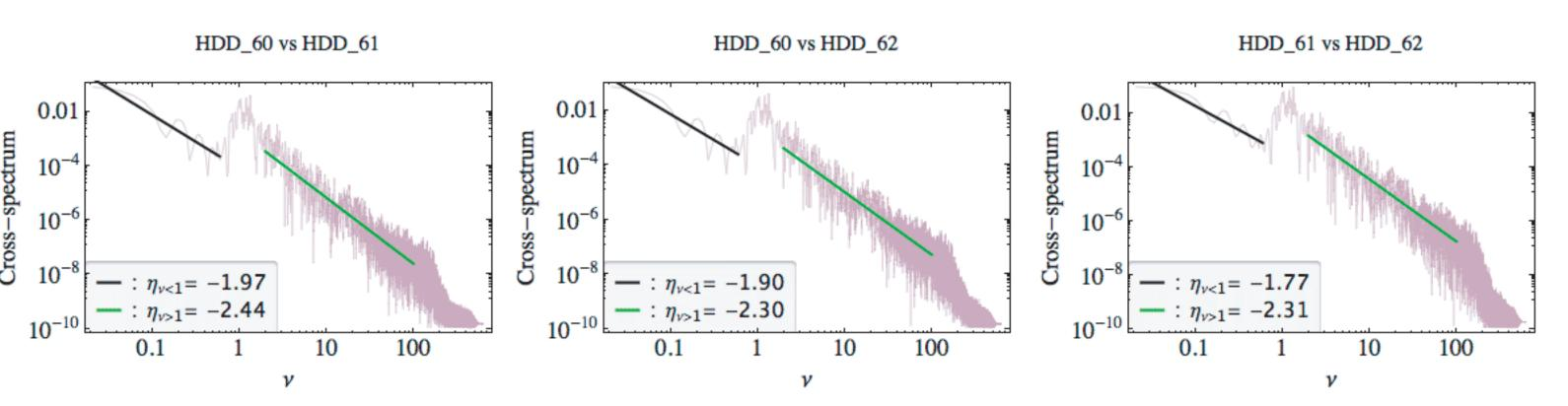
Figure 7: Cross-spectra computed between the pore pressure signals recorded at different depths (Figure 3). The curves exhibit the same behavior illustrated in Figure 5, where a sharp discontinuity is observed at 1Hz and attenuation follows a power law for frequencies < 1Hz and from 2 Hz - 100 Hz. The exponents characterizing the power law attenuation of the spectral curves have the same order of magnitude than those reported in Figure 5.
